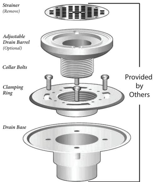
An exploded view of a typical shower flanged drain assembly is shown on the left for your reference. This assembly can be made from PVC, cast iron or other composite materials.
